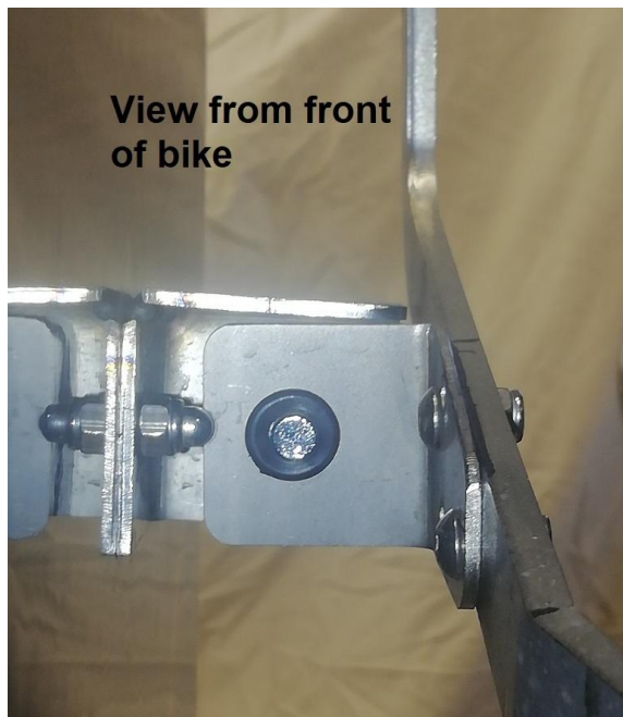
Bracket fitted to support arm
